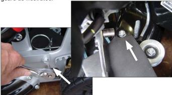
Pull the shift lever towards the "LO" speed setting of the transmission. Rotate the cover clockwise for removal.
