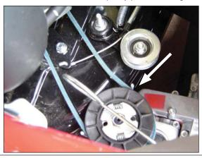
**STEP 4**Pull out the belt under the deck as illustrated.
