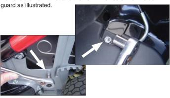
Pull the shift lever towards the "LO" speed setting of the transmission. Lift up on the shift lever at the same time as lifting the cover. The cover slides off towards the right side.
