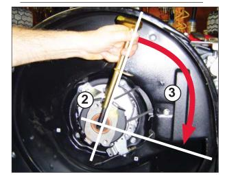
Install the Allen wrench with the short end into the screw and extend it with the combination wrench.
