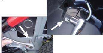
Pull the shift lever towards the "LO" speed setting of the transmission. Lift up on the shift lever at the same time as lifting the cover. The cover slides off towards the right side.
