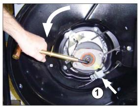
Step 6 Remove the clutch from the crankshaft.
