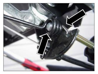
The combination of the bail going past the Bail Stop Spring too easily and a cable that has developed a kink will eventually cause the drive cable to fail at the ball.
