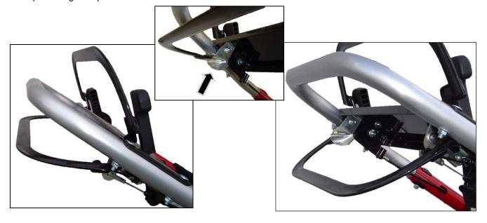
The one side effect if the Bail Stop Spring is adjusted too loosely is that the bail falls down too easily and it becomes less operator friendly. HOWEVER we have discovered a second side effect that it can cause premature failure of the drive cable for the transmission.
