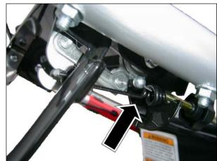
If the cable ball and the hook are "stuck together" the cable can "kink".
