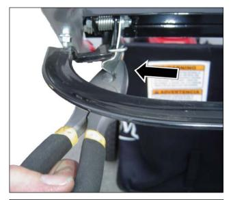
As of 2011 production we have redesigned the end of the cable to avoid the kinking.
