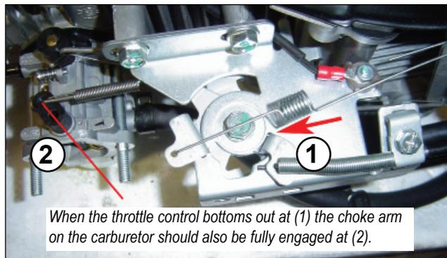
When the throttle control bottoms out at (1) the choke arm on the carburetor should also be fully engaged at (2).
