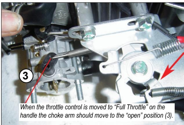
When the throttle control is moved to "Full Throttle" on the handle the choke arm should move to the "open" position (3).
