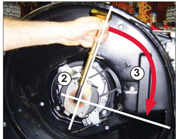
2. Install the Allen wrench with the short end into the screw and extend it with the combination wrench.
