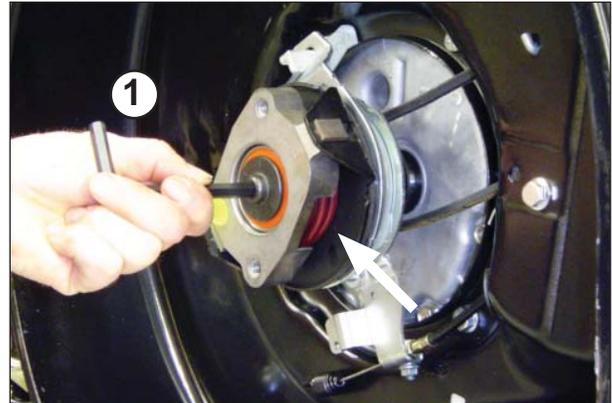
1. Use the Allen Wrench as illustrated - Tighten the screw as much as possible with your hand. The screw will turn with difficulty for a few turns and come to a distinct stop. This process compresses the spring on the lower clutch part.
